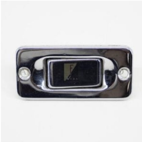
SWITCH (INTERIOR LIGHTS) ON CONSOLE (FV/ HK/ EXC/ FACEL II )
